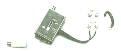
C. Connect the twin-lead wire from the TV/GAME Switch Box to the VHF antenna terminals on your television set.
